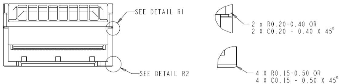
Figure 3-7: OSFP corner radius
